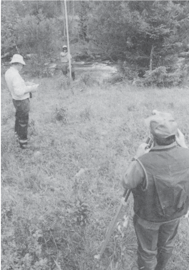
Figure 49. Good location for level setup.
