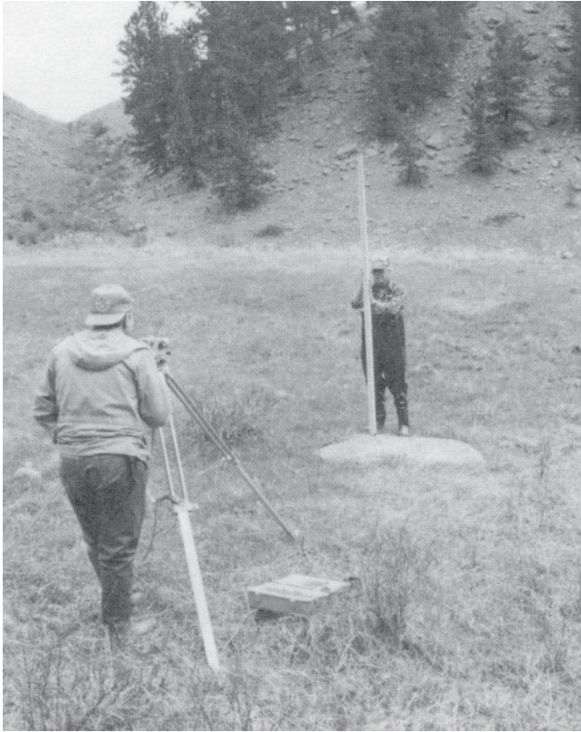
Figure 34. Shooting the elevation of the benchmark.
