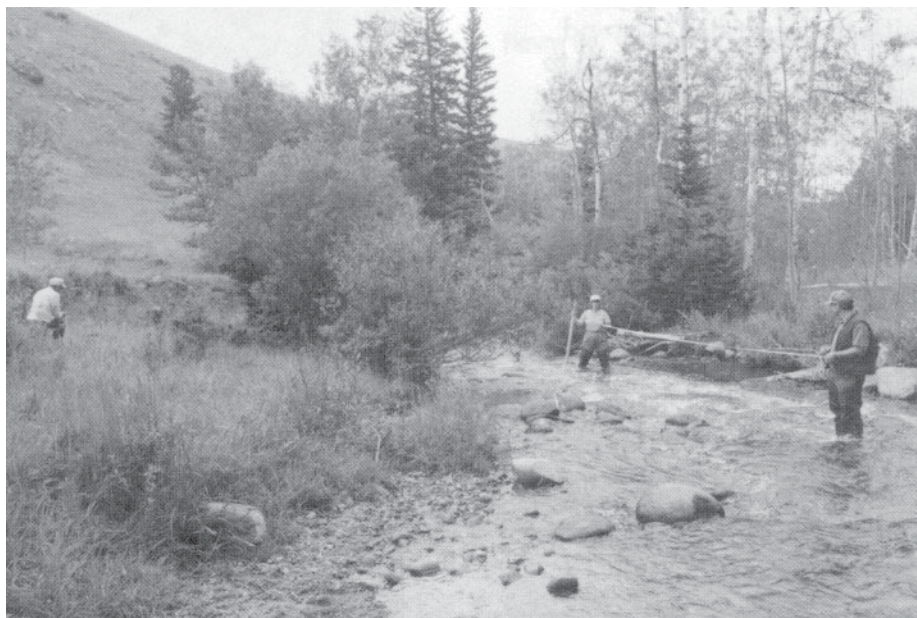
Figure 50. Measuring along the channel centerline and staking.
